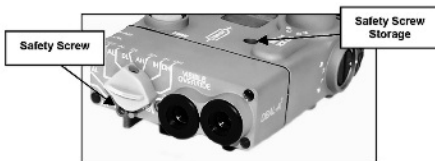
Figure 3-3 Safety Screw Installed (shown in Training Mode)
