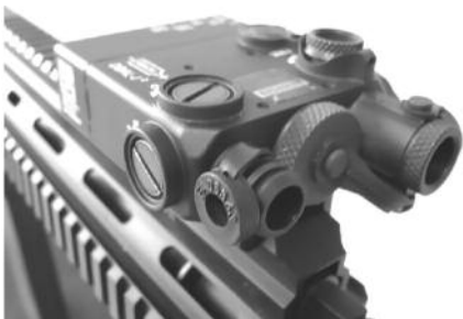
Figure 3-12 DBAL-I 2 Top Mounted on M4/M16A
