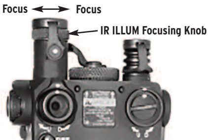
Figure 3-7 The IR ILLUM Focusing Knob
