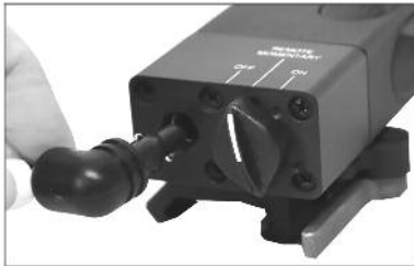
Figure 3-2 Remote Cable Switch Location
