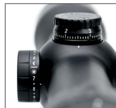
Reticle illumination is powered by a 3-volt CR 2032 battery. The battery is located in the illumination knob and can be accessed by unscrewing the cover. To insert a new battery, screw the battery compartment open on the left side. Press on one side of the battery to lift and remove. Install the new battery with the flat side (+) up. If you are planning on not using the riflescope for an extended period, it is advisable to remove the battery.
